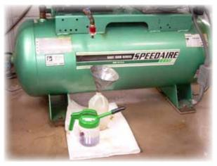
This Speedair reciprocating compressor is equipped with an Esco Oil Sight Glass. The Oil Safe container holds Monolec 6404 for the compressor.
