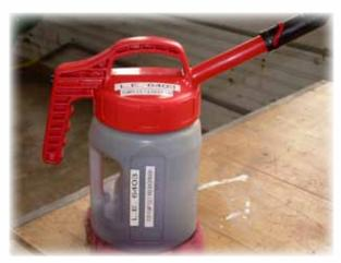
This Oil Safe container holds Monolec 6403 for the DeLaval pumps. It is stored near the pumps.
